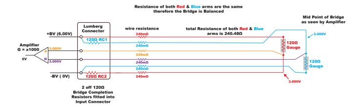
Another option is to place the completion resistors as close to the gauges as possible, this leads to the same result as above. Fylde part number FE-349-BA offers a small box containing the completion resistors (240R standard, other values available on request) and 2 connectors to interface to the gauges (plug type Weald Electronics SM2SN).
