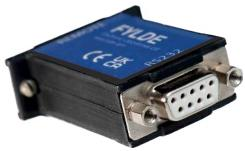
The FE-390-IF is a compact module that provides remote control of compatible Fylde modules. The unit connects to the rear of racks fitted with remote enabled 15-way D connectors and is powered by the rack. A 2nd D connector (9-way) provides a standard RS232 link to a PC. ASCII commands sent from a terminal program such as Hyperterminal or RealTerm set the parameters of individual or multiple modules in the rack. Settings can also be retrieved and viewed remotely from modules.
